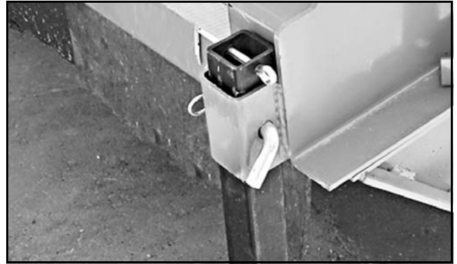
Figure 44. Front Stands Installed
